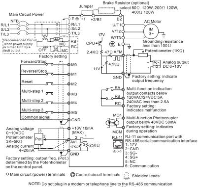
port, permanent damage may result. Pins 1&2 are the power sources for the optional copy keypad and should not be used while using RS-485 communication.
