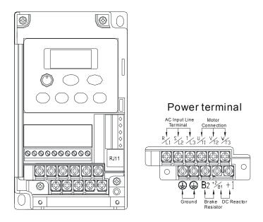
Power Terminal: Torque: 12 kgf-cm (10 lbf-in) Wire Gauge: 14-20 AWG (2.1-0.5mm<sup>2</sup>) Wire Type: Copper only, 75°C
