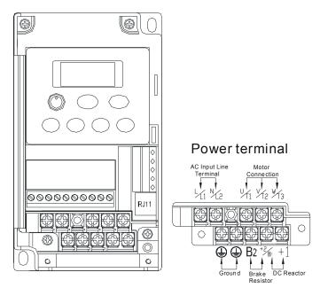
Power Terminal: Torque: 12 kgf-cm (10 lbf-in) Wire Gauge: 14-20 AWG (2.1-0.5mm<sup>2</sup>) Wire Type: Copper only, 75°C
