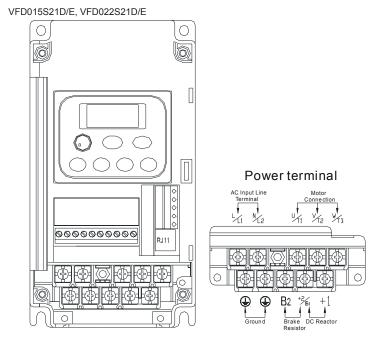
Power Terminal: Torque: 20 kgf-cm (17.4 lbf-in) Wire Gauge: 10-18 AWG (5.3-0.8mm<sup>2</sup>) Wire Type: stranded copper only, 75°C
